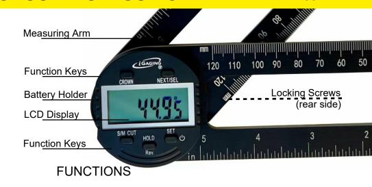
**Battery:** CR2032; 1 piece. Slide the battery holder out on the left of the LCD Display; insert a CR2032 battery with "+" side facing up/out; re-insert the battery holder in place to power the gauge on. (In some markets, the battery is pre-installed for convenience.)
